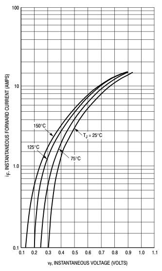
Figure 1. Typical Forward Voltage
