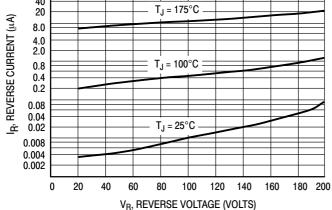
$^\star$  The curves shown are typical for the highest voltage device in the voltage grouping. Typical reverse current for lower voltage selections can be estimated from these same curves if applied V<sub>R</sub> is sufficiently below rated V<sub>R</sub>.
