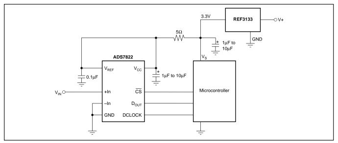
FIGURE 6. Basic Data Acquisition System 1.
