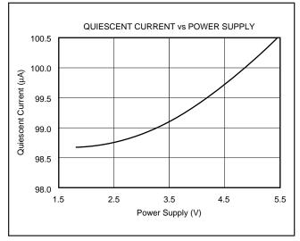
FIGURE 3. Supply Current vs Supply Voltage.
