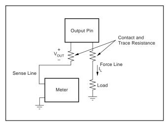
FIGURE 4. Accurate Load Regulation of REF31xx.
