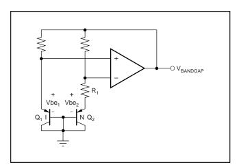
FIGURE 1. Simplified Schematic of Bandgap Reference.
