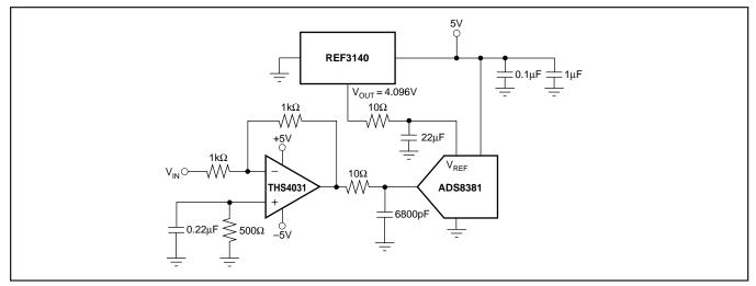
FIGURE 8. REF3140 Provides an Accurate Reference for Driving the ADS8381.
