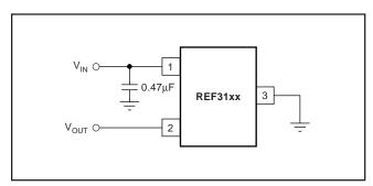
FIGURE 2. Typical Connections for Operating REF31xx.
