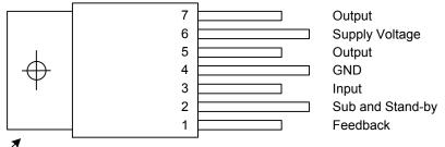
ZTAB Connected to Pin 4
