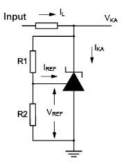
Figure 2. Test circuit for V<sub>KA</sub> > V<sub>REF</sub>
