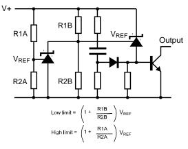
Over voltage / under voltage protection circuit
