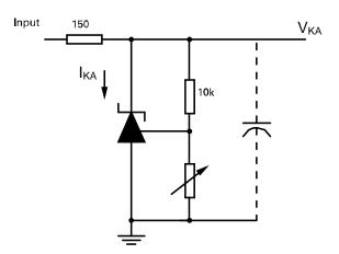
$V_{REF} < V_{KA} < 20V, \ I_{KA} = 10mA, \ T_A = +25^{\circ}C$  Test Circuit for Stability Boundary Conditions
