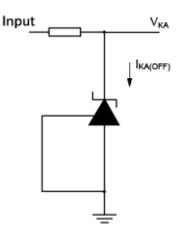
Figure 3. Test circuit for off state current
