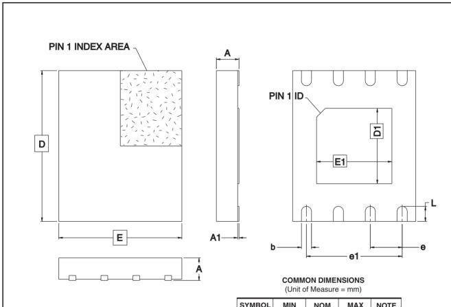
Note: Soldering the large thermal pad is optional, but not recommended.
