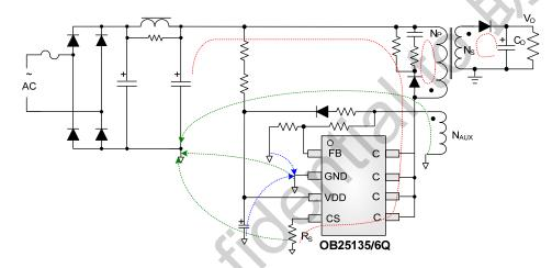
Fig.5 Flyback Schematic with OB25135/6Q
