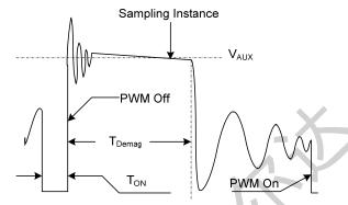
Figure 2 Auxiliary voltage waveform
