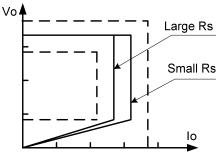
Figure 3. Adjustable output power by changing Rs
