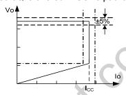
Figure.1. Typical CC/CV Curve
