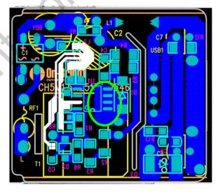
Fig.6 Recommend PCB Layout of OB25135/6Q
