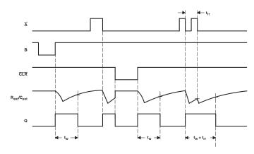
Figure 2. Input/Output Timing Diagram
