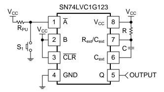
Figure 10. Typical Application of the SN74LVC1G123
