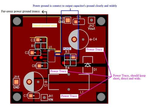
(AX5201 PCB Layout -Top View)
