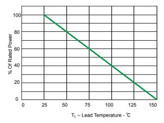
Fig 2.Power Derating Curve
