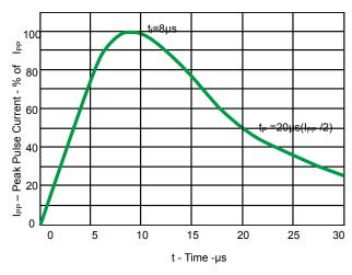
Fig 1.Pulse Waveform
