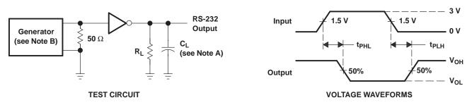
NOTES: A. C<sub>L</sub> includes probe and jig capacitance.
