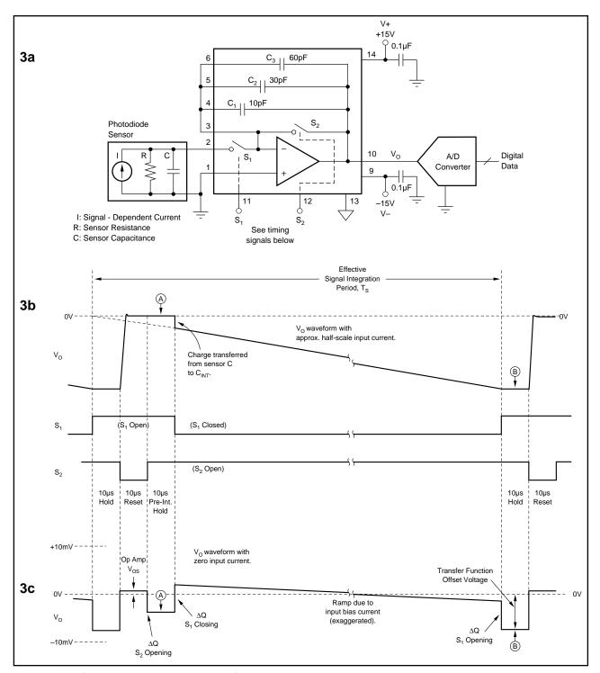
FIGURE 3. Switched-Input Measurement Technique.
