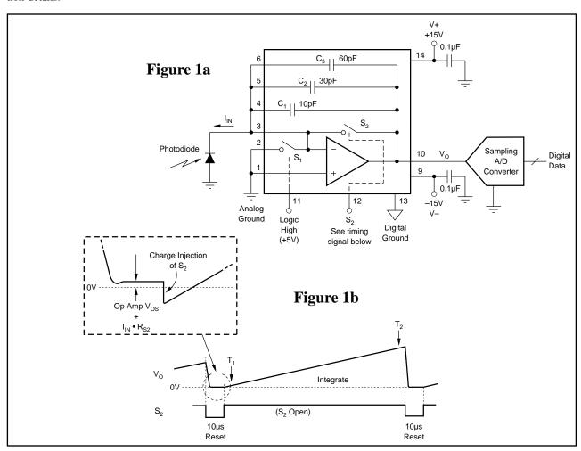
FIGURE 1. Reset-and Integrate Connections and Timing.
