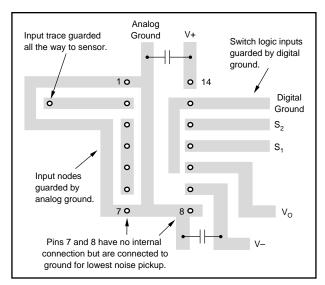
FIGURE 4. Circuit Board Layout Techniques.
