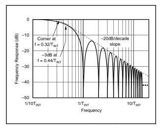
FIGURE 5. Frequency Response of Integrating Converter.
