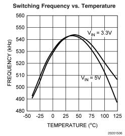
**Typical Performance Characteristics** Unless otherwise specified, the following conditions apply:  $V_{IN} = AVIN = PVIN = 5V$ ,  $T_J = 25$ °C. (Continued)
