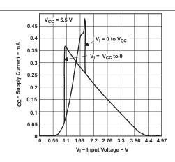
Figure 2. Supply Current vs Input Voltage
