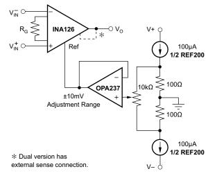
Figure 19. Optional Trimming of Output Offset Voltage
