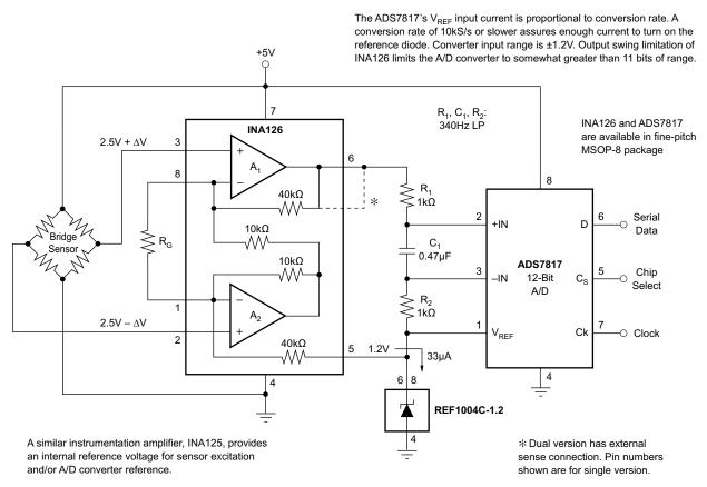
Figure 25. Bridge Signal Acquisition, Single 5-V Supply
