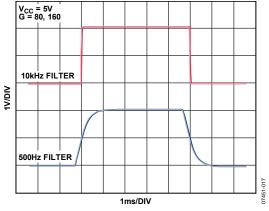
Figure 17. Large Signal Step Response
