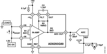
Figure 21. Measuring Current Through a Shunt Resistor (Filter Is Set to 500 Hz)
