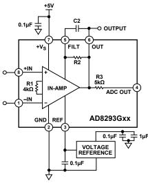
Figure 20. Operating on a Single Supply Using an External Voltage Reference (The Output Can Be Used Without an Antialiasing Filter if the Signal Bandwidth Is <10 Hz)
