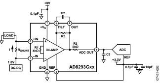
Figure 2. Measuring Current Using the AD8293G80/AD8293G160
