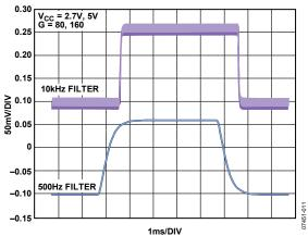
Figure 15. Small Signal Step Response
