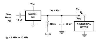
**Figure 3. Total Harmonic Distortion Test Circuit**
