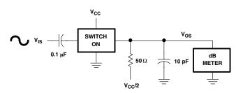
Figure 2. Frequency-Response Test Circuit
