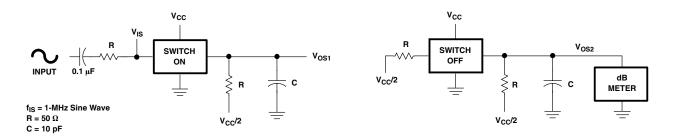
Figure 1. Crosstalk Between Two Switches Test Circuit
