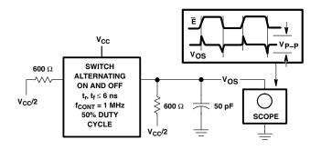
Figure 4. Control-to-Switch Feedthrough Noise Test Circuit
