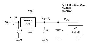
Figure 5. Switch OFF Signal Feedthrough Test Circuit
