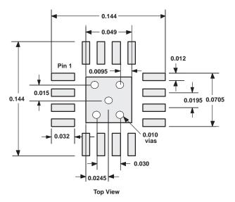
Figure 50. PowerPAD PCB Etch and Via Pattern
