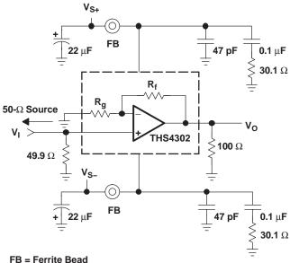
Figure 44. Wideband, Noninverting **Gain Configuration**
