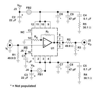
Figure 52. Typical THS4302 EVM Circuit Configuration
