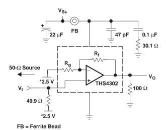
Figure 45. DC-Coupled Single Supply Operation
