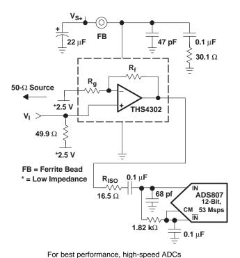
Figure 47. Driving an ADC With a Single-Ended Input
