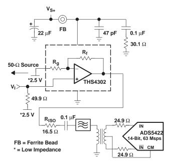
Figure 46. Driving an ADC Via a Transformer
