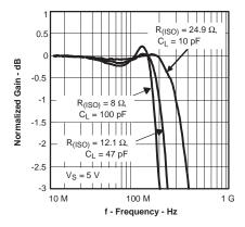
Figure 48. Driving Capacitive Loads
