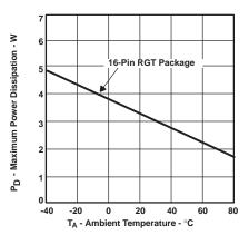
$\theta_{JA}$  = 39.5°C/W for 16-Pin MSOP (RGT)  $T_{J}$  = 150°C, No Airflow
