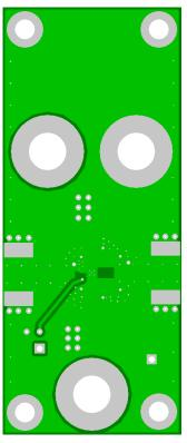
Figure 55. THS4302EVM Board Layout (Bottom Layer)
