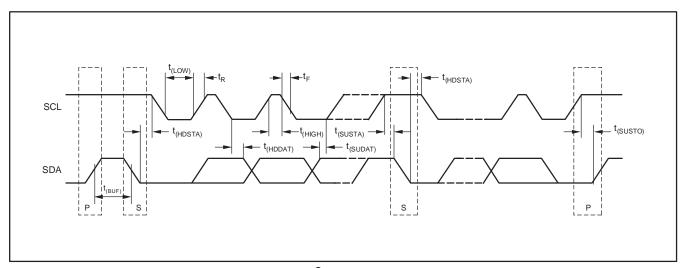
Figure 5. I<sup>2</sup>C Timing Diagram
