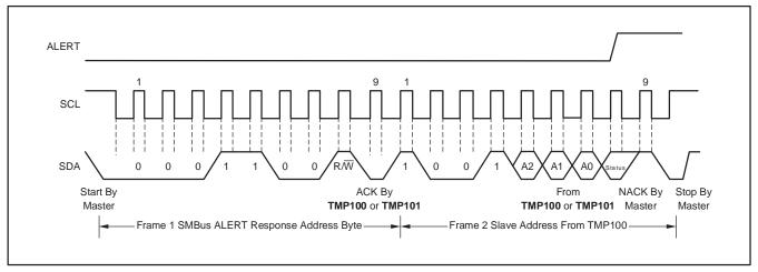
Figure 8. Timing Diagram for SMBus ALERT
