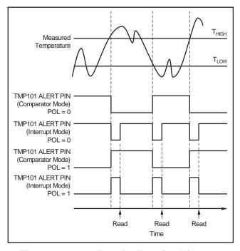
Figure 4. Output Transfer Function Diagrams
