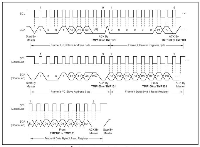
Figure 7. I<sup>2</sup>C Timing Diagram for Read Word Format
