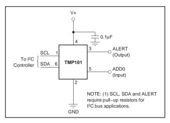
Figure 1. Typical Connections of the TMP101
