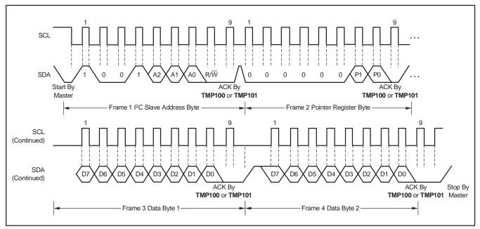
Figure 6. I<sup>2</sup>C Timing Diagram for Write Word Format
