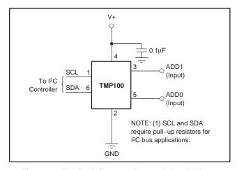
Figure 2. Typical Connections of the TMP100
