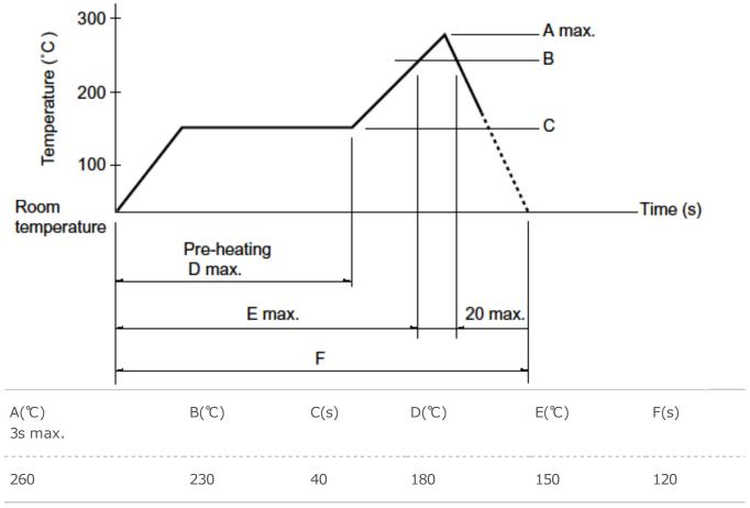
(1) The condition mentioned above is the temperature on the mounting surface of a PC board. There are cases where the PC board's temperature greatly differs from that of the switch, depending on the PC board's material, size, thickness, etc. The above-stated conditions shall also apply to switch surface temperatures.
