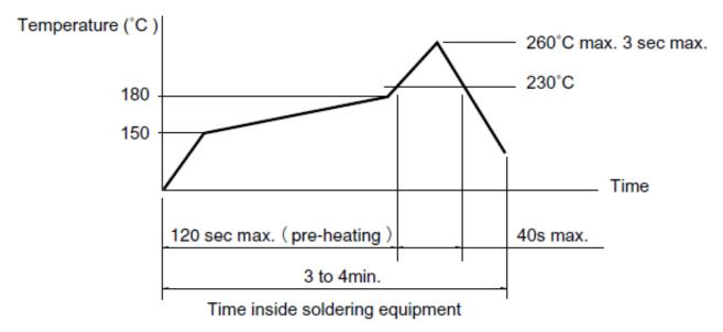
(1) The above temperature shall be measured of the top of switch. There are cases where PC board's temperature greatly differs from that of the switch, depending on the material, size, thickness of PC board's and others. Care, should be taken to prevent the switch's surface temperature from exceeding  $260^{\circ}$ C.
