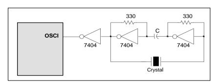
Figure 6-19 Serial Mode Crystal/Resonator Circuit Diagram
