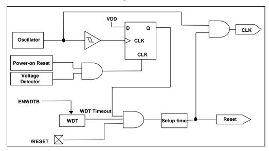
Figure 6-8 Controller Reset Block Diagram
