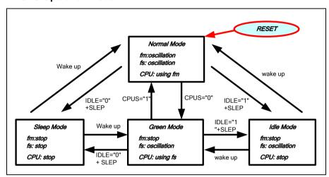
Figure 6-3 CPU Operation Mode Diagram
