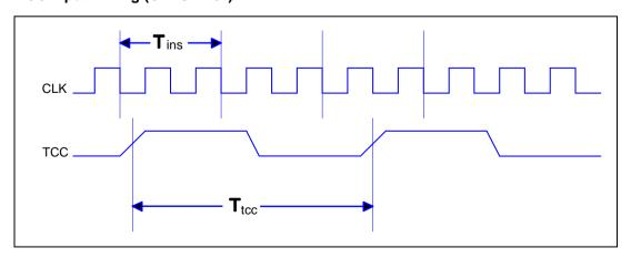
Figure 10-1c TCC Input Timing Diagram
