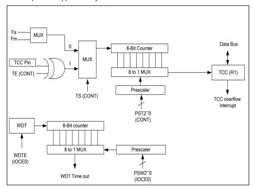
Figure 6-3 TCC and WDT Block Diagram
