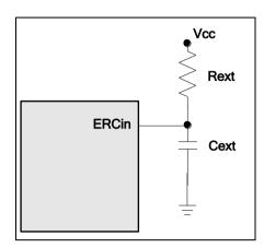
Figure 6-22 External RC Oscillator Mode Circuit
