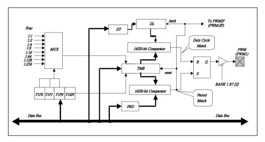
Figure 6-14 Functional Block Diagram of 16/20-bit PWM (merged from two 8/10 bits)
