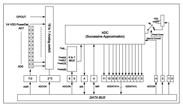
Figure 6-10 Analog-to-Digital Conversion Functional Block Diagram
