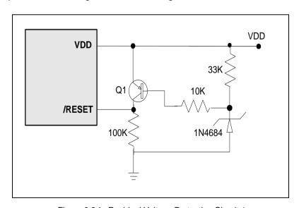
Figure 6-24 Residual Voltage Protection Circuit 1
