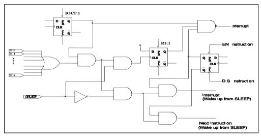
Figure 6-7 Port 5 Block Diagram with Input Change Interrupt/Wake-up
