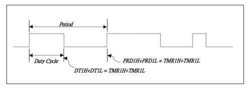
Figure 6-13 PWM Output Timing
