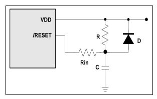
Figure 6-23 External Power-on Reset Circuit
