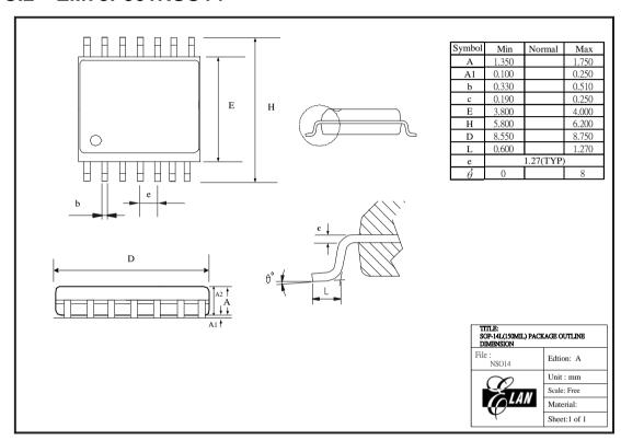
Figure C-2 EM78P301N 14-pin SOP Package Type
