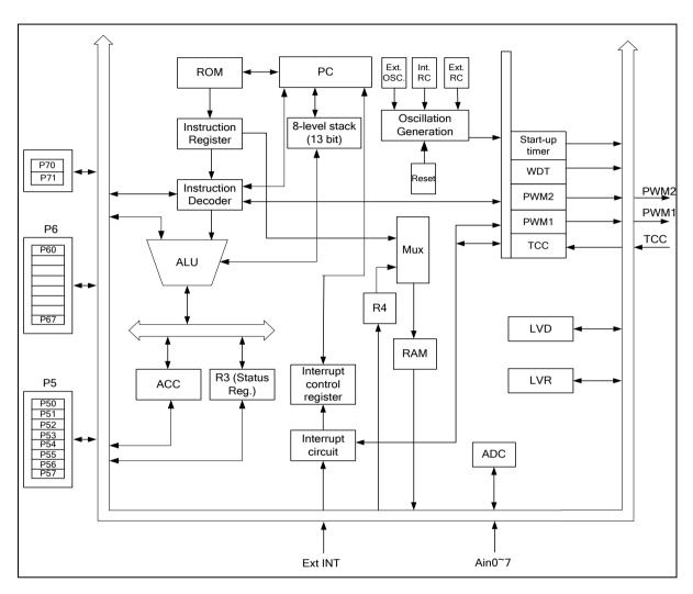
Figure 5-1 EM78P301N Block Diagram
