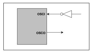
Figure 6-17 External Clock Input Circuit
