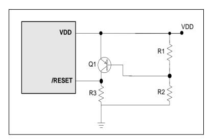
Figure 6-25 Residual Voltage Protection Circuit 2
