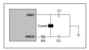
Figure 6-18 Crystal/Resonator Circuit
