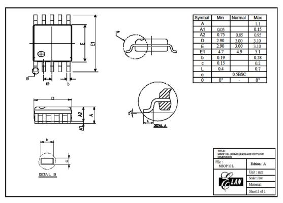
Figure C-9 EM78P301N 10-pin MSOP Package Type
