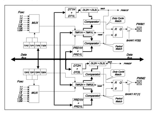
Figure 6-12 PWM System Block Diagram
