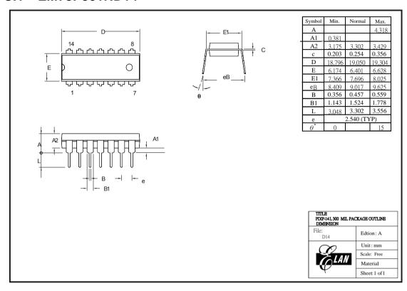
Figure C-1 EM78P301N 14-pin PDIP Package Type
