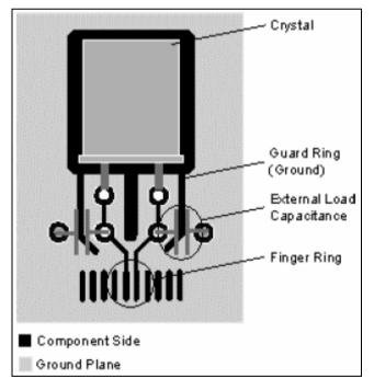
Figure 6-21 Parallel Mode Crystal/Resonator Circuit Diagram
