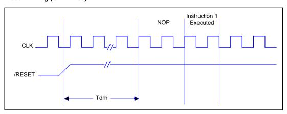
Figure 10-1b Reset Timing Diagram
