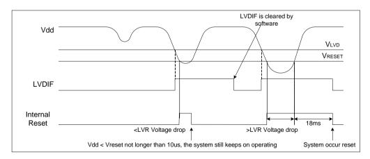
Figure 6-26 LVD/LVR Waveform
