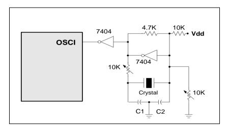
Figure 6-20 Parallel Mode Crystal/Resonator Circuit Diagram
