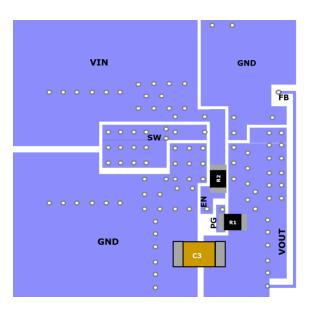
FIG.60 Recommendation Layout (Bottom)
