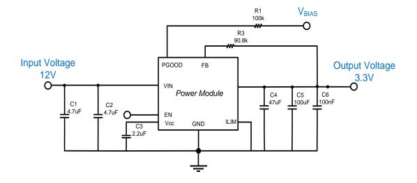
FIG.55 REFERENCE CIRCUIT FOR GENERAL APPLICATION
