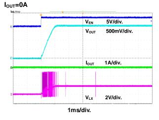
Figure 14. Power On through EN Waveform
