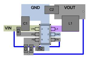
Figure 19. Recommended Layout Diagram
