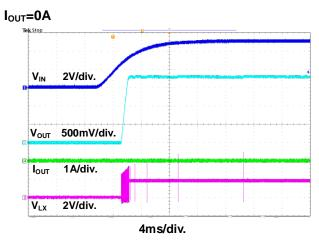
Figure 10. Power On through VIN Waveform
