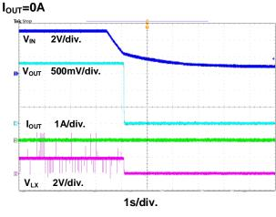
Figure 12. Power Off through VIN Waveform
