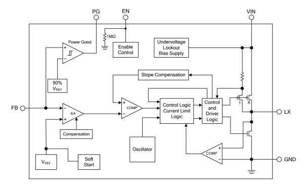
Figure 3. Block Diagram of FP6373A
