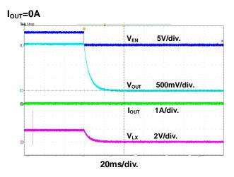
Figure 16. Power Off through EN Waveform
