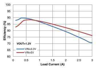
Figure 4. Efficiency vs. Load Current
