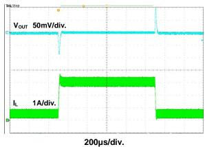
Figure 18. Load Transient Waveform
