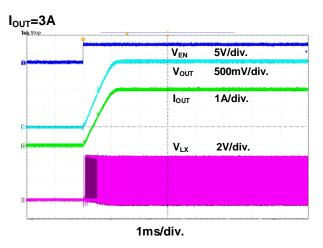
Figure 15. Power On through EN Waveform
