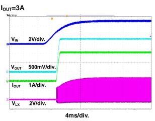
Figure 11. Power On through VIN Waveform
