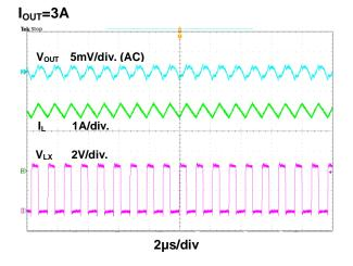
Figure 9. Steady State Waveform
