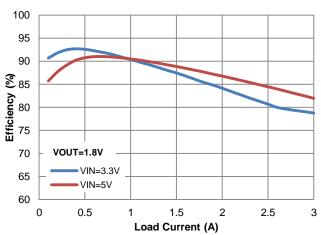
Figure 5. Efficiency vs. Load Current
