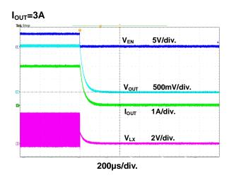
Figure 17. Power Off through EN Waveform
