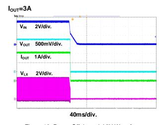
Figure 13. Power Off through VIN Waveform
