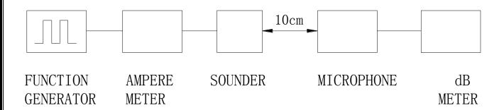
In the measuring test, buzzer is placed as follows:
