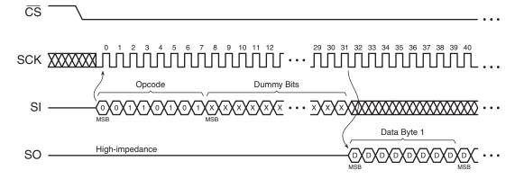
Figure 25-9. Read Security Register (Opcode 77h)
