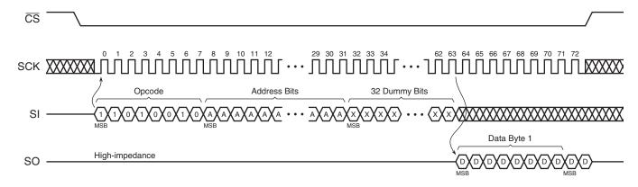
Figure 25-5. Buffer Read (Opcode D4h)
