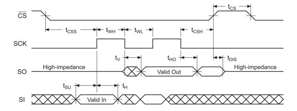
Figure 22-2. Waveform 2 = SPI Mode 3 Compatible
