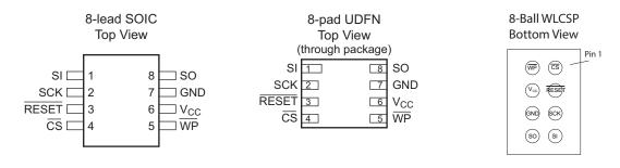
Note: 1. The metal pad on the bottom of the UDFN package is not internally connected to a voltage potential. This pad can be a "no connect" or connected to GND.
