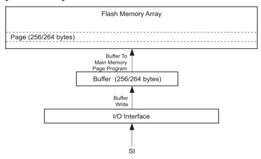
Figure 23-2. Buffer Write
