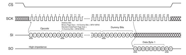
Figure 25-6. Buffer Read - Low Frequency (Opcode D1h)
