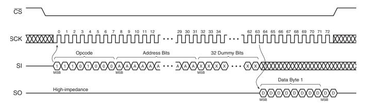
Figure 25-2. Continuous Array Read (Opcode 0Bh)
