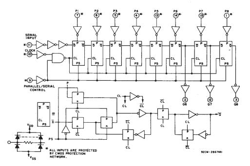
Fig. 2 - Logic diagram for CD40218.
