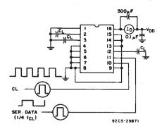
Fig. 10 - Dynamic power dissipation test circuit.
