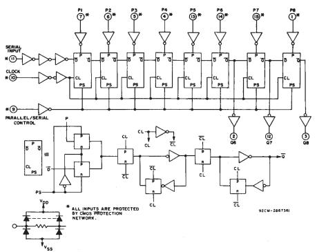
Fig. 1 - Logic diagram for CD4014B.
