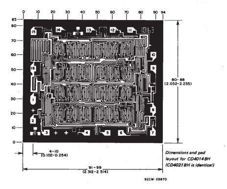
Dimensions in perentheses are in millimeters and are derived from the basic inch dimensions as indicated. Grid graduations are in mils ( $10^{-3}$  inch).
