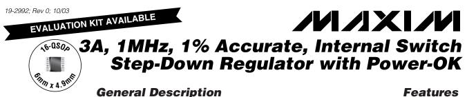
The MAX8505 step-down regulator operates from a 2.6V to 5.5V input and generates an adjustable output voltage from 0.8V to 0.85 × VIN at up to 3A. With a 2.6V to 5.5V bias supply, the input voltage can be as low as 2.25V.
