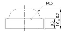
For reflow soldering (Propose)
