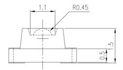
For reflow soldering (propose)
