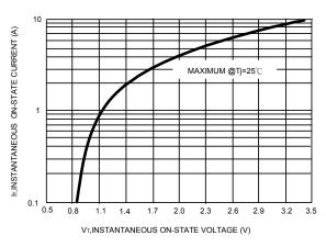
Figure 5. Typical On-State Characteristics
