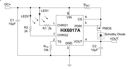
\*The charge current  $I_{O(REG)} = V_{CS}/R_{SET}$  ( $V_{CS}$  is usually 200mV). Note that OFF indicates the open-drain transistor is turned off.
