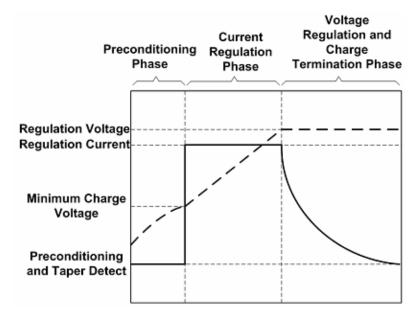
Figure 2: Typical Charge Profile
