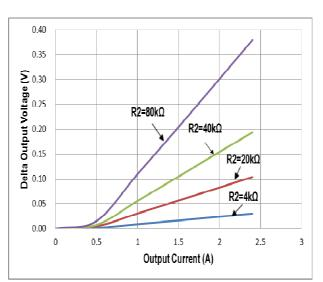
$V_{OUT} = [(1 + \frac{R_{FB1}}{R_{FB2}}) \times V_{FB}] + [R_{FB1} \times (\frac{V_{SEN}}{16.6K} - 1uA)]$
