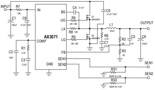
Note: If output only 1 port, the other Sense pin need connect with GND.
