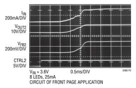
Figure 4. Start-Up Waveforms
