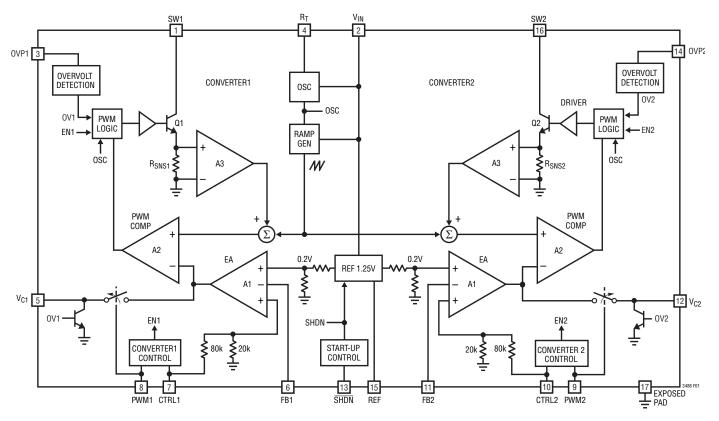
Figure 1. LT3486 Block Diagram
