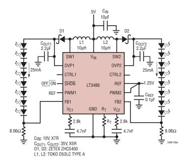
Figure 6a. 5V to 8/8 White LEDs
