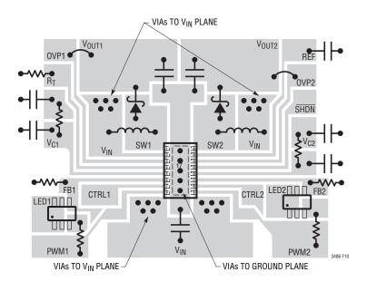
Figure 10. Recommended Layout for LT3486
