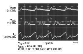
Figure 2. Switching Waveforms
