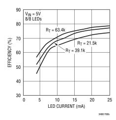
Figure 6b. Efficiency Comparison for Different R<sub>T</sub> Resistors
