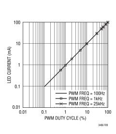
Figure 9. LED Current Variation vs PWM Duty Cycle
