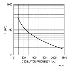
Figure 5. Timing Resistor (R<sub>T</sub>) Value
