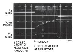
Figure 3a. Transient Response of Switcher 1 with LED1 Disconnected from the Output
