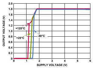
FIGURE 5. OUTPUT VOLTAGE vs SUPPLY VOLTAGE
