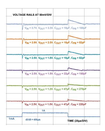
**FIGURE 9. LOAD TRANSIENT RESPONSE**
