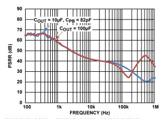
FIGURE 13. PSRR vs FREQUENCY FOR VARIOUS OUTPUT CAPACITORS (I<sub>OUT</sub> = 100mA)
