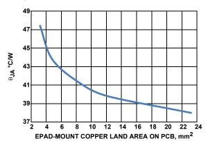
FIGURE 16. 3mmx3mm 10-PIN DFN ON 4-LAYER PCB WITH THERMAL VIAS  $\theta_{
