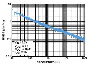
FIGURE 15. OUTPUT NOISE SPECTRAL DENSITY
