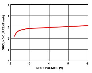
FIGURE 8. GROUND CURRENT vs SUPPLY VOLTAGE
