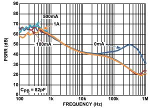
FIGURE 12. PSRR vs FREQUENCY FOR VARIOUS LOAD CURRENTS
