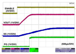
FIGURE 11. ENABLE START-UP (C<sub>SS</sub> = 2.2nF)
