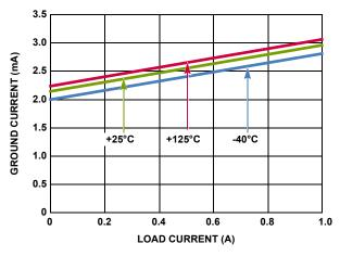
FIGURE 7. GROUND CURRENT vs LOAD CURRENT
