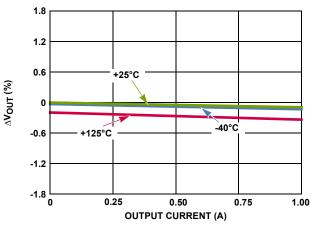
FIGURE 6. OUTPUT VOLTAGE vs OUTPUT CURRENT
