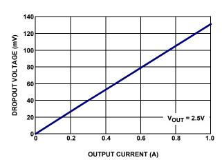
FIGURE 2. DROPOUT vs LOAD CURRENT
