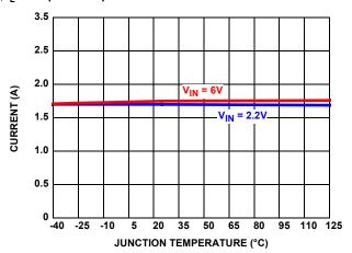
FIGURE 10. CURRENT LIMIT vs TEMPERATURE (V<sub>OUT</sub> = 0V)
