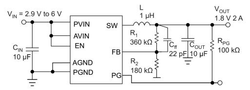
Figure 10. TPS62067-Q1 Adjustable 1.8-V Output-Voltage Configuration
