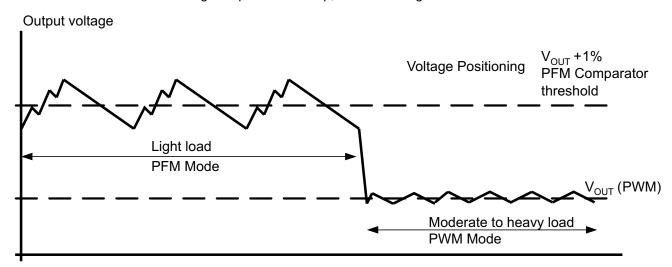
Figure 8. Power Save Mode Operation with automatic Mode transition
