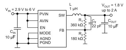
Figure 9. TPS62065-Q1 Adjustable 1.8-V Output-Voltage Configuration
