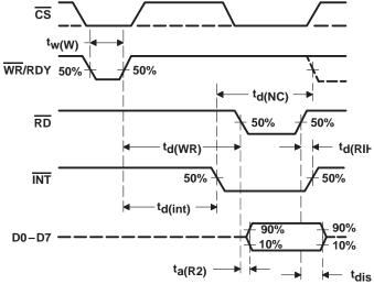
Figure 3. Write-Read-Mode Waveforms [MODE High and t<sub>d(WR)</sub> > t<sub>d(int)</sub>]
