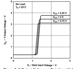
Figure 9. Y Output Voltage vs Data Input Voltage
