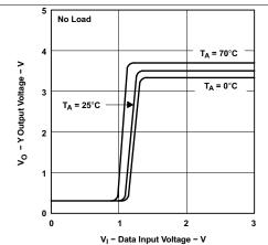
Figure 10. Y Output Voltage vs Data Input Voltage
