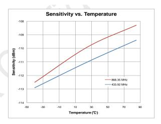
Figure 6. Sensitivity vs. Temperature,  $F_{RF}$  = 433.92 / 868.35 MHz, FSK,  $V_{DD}$  = 3.3 V, SR = 1 ksps, BER = 0.1%
