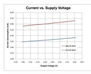
Figure 3. Current vs. Voltage,  $F_{RF}$  = 433.92 / 868.35 MHz, OOK, SR = 1 ksps
