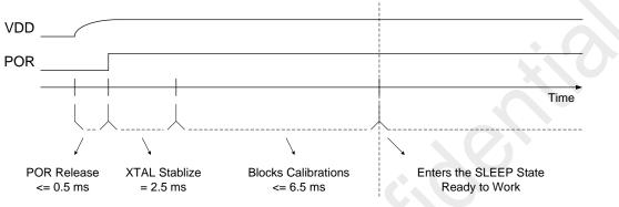
Figure 16. Power-Up Sequence Timing
