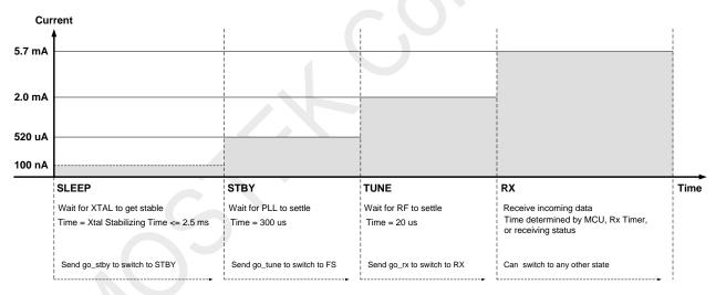
Figure 18. Timing and Power from SLEEP to RX state
