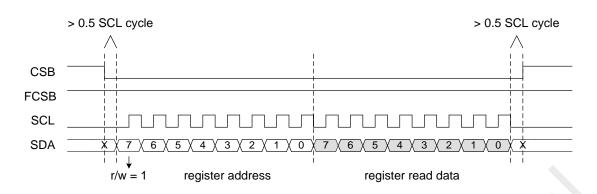
Figure 13. SPI Read Register Timing
