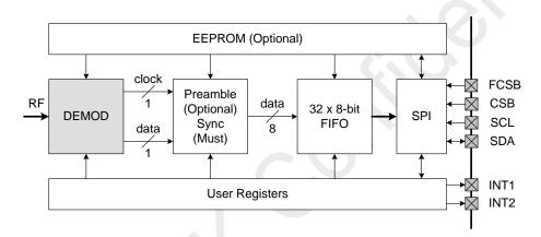
Figure 22. Data Path of Buffer Mode
