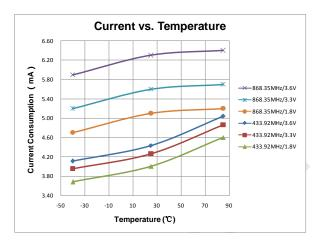
Figure 4. Current vs. Temperature,  $F_{RF}$  = 433.92 / 868.35 MHz, FSK, SR = 1 ksps
