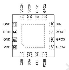
Figure 2. CMT2219A Pin Assignments
