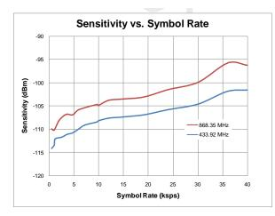
Figure 7. Sensitivity vs. SR,  $F_{RF}$  = 433.92 / 868.35 MHz, OOK,  $V_{DD}$  = 3.3 V, BER = 0.1%
