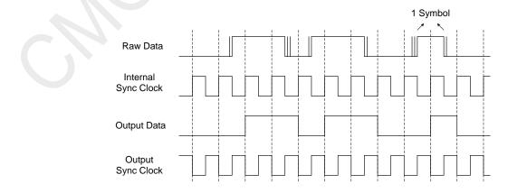
Figure 21. Demodulated Data and Sync Clock Timing Characteristics
