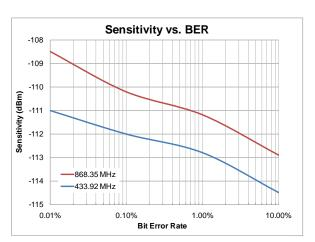
Figure 8. Sensitivity vs. BER,  $F_{RF}$  = 433.92 / 868.35 MHz,  $V_{DD}$  = 3.3 V, SR = 1 ksps
