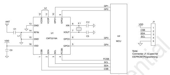
Figure 1. CMT2219A Typical Application Schematic
