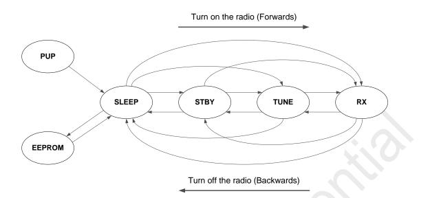
Figure 17. Device Operating State Machine
