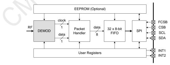
Figure 23. Data Path of Packet Mode
