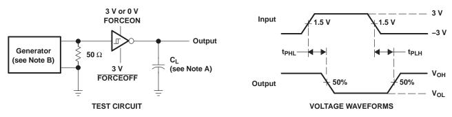
NOTES: A. C<sub>1</sub> includes probe and jig capacitance.
