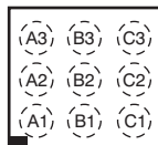
YFF Package 9-Pin DSBGA Top View
