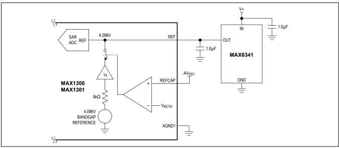
Figure 18. External Reference Operation
