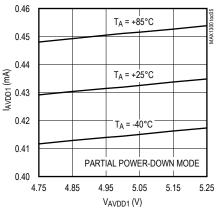
DIGITAL SUPPLY CURRENT vs. DIGITAL SUPPLY VOLTAGE
