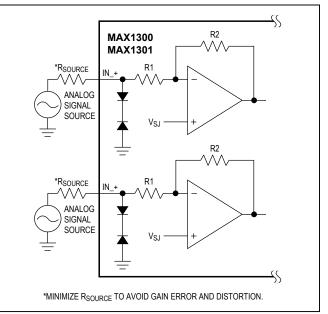
Figure 6. Simplified Analog Input Circuit
