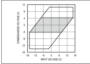
Figure 11. Common-Mode Voltage vs. Input Voltage (FSR = 12 x V<sub>RFF</sub>)
