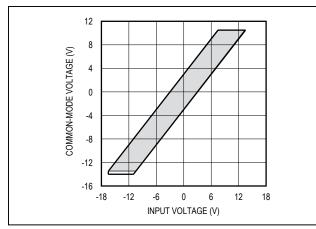
Figure 9. Common-Mode Voltage vs. Input Voltage (FSR = 3 x V<sub>REF</sub>)
