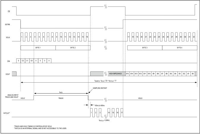
Figure 3. External Acquisition-Mode Conversion (Mode 1)
