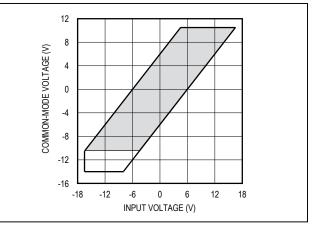
Figure 10. Common-Mode Voltage vs. Input Voltage (FSR = 6 x V<sub>REF</sub>)
