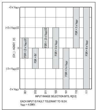
Figure 7. Single-Ended Input Voltage Ranges
