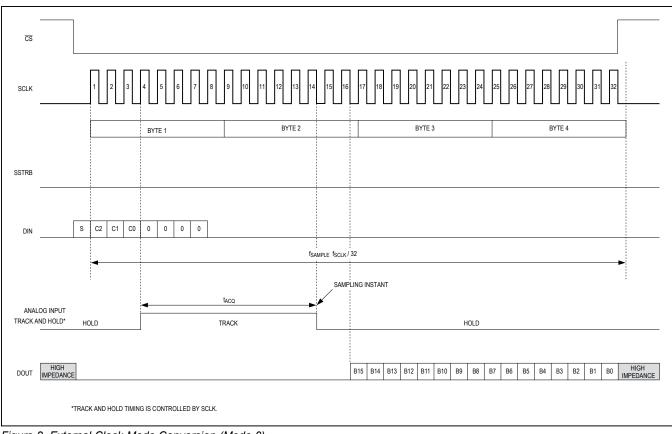
Figure 2. External Clock-Mode Conversion (Mode 0)
