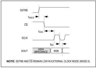
Figure 16. DOUT and SSTRB Timing
