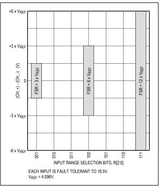
Figure 8. Differential Input Voltage Ranges
