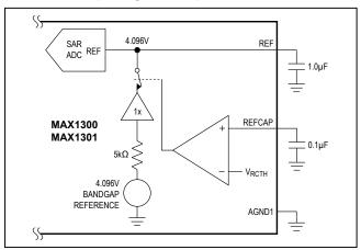
Figure 17. Internal Reference Operation
