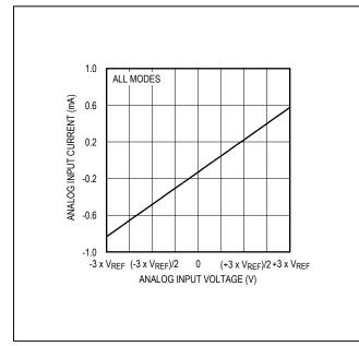
Figure 5. Analog Input Current vs. Input Voltage
