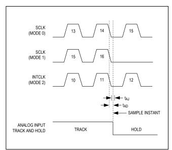
Figure 21. Aperture Diagram
