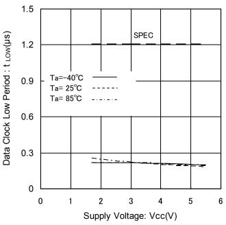
Figure 15. Data Clock Low Period vs Supply Voltage
