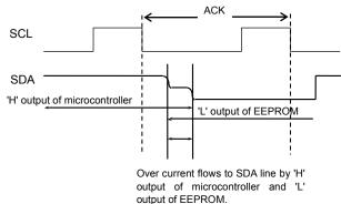
Figure 45. I/O Circuit Diagram
