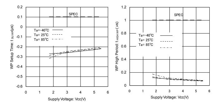
Figure 32. WP Setup Time vs Supply Voltage
