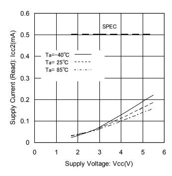
Figure 11. Supply Current (Read) vs Supply Voltage (f<sub>SCL</sub>=400kHz)
