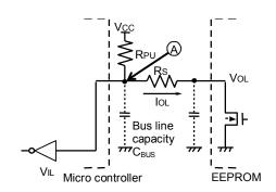
Figure 47. I/O Circuit Diagram
