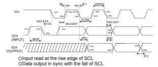
Figure 2-(a). Serial Input / Output Timing
