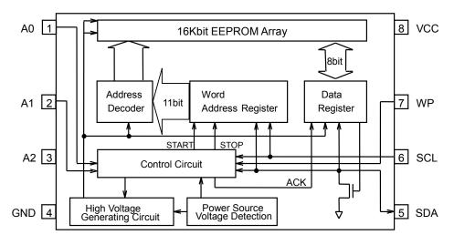
Figure 3. Block Diagram
