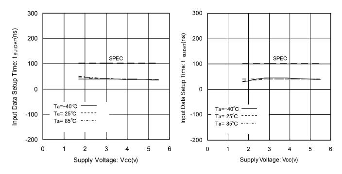
Figure 20. Input Data Setup Time vs Supply Voltage (HIGH)
