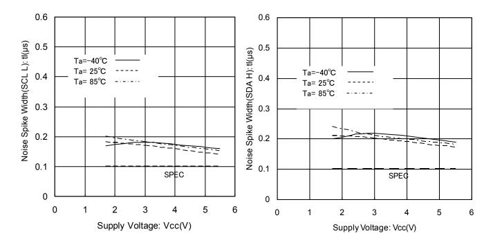
Figure 28. Noise Spike Width vs Supply Voltage (SCL L)
