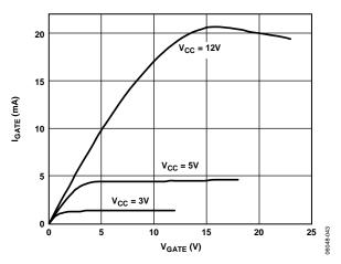
Figure 12. Gate Pull-Down Current vs. Gate Voltage
