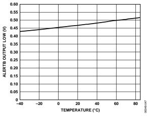
Figure 30. ALERTB Output Low Voltage vs. Temperature @ 1 mA
