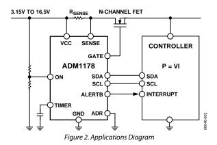
A 12-bit ADC can measure the current seen in the sense resistor, as well as the supply voltage on the VCC pin. An alert output can be set to trigger when the ADC current reading exceeds a programmed overcurrent limit threshold.
