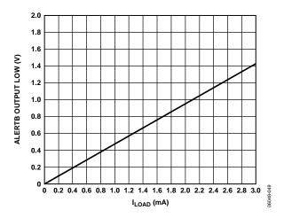
Figure 32. ALERTB Output Low Voltage vs. Load Current
