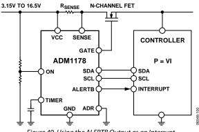
Figure 49. Using the ALERTB Output as an Interrupt
