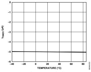
Figure 19. Timer Pull-Up Current (Initial Cycle) vs. Temperature
