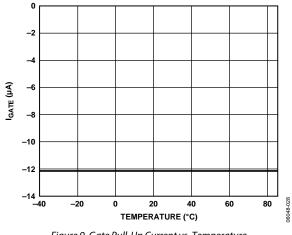
Figure 9. Gate Pull-Up Current vs. Temperature
