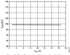
Figure 22. Circuit Breaker Limit Voltage vs. Supply Voltage
