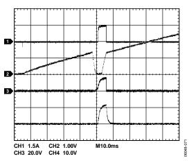
Figure 45. Overcurrent Condition at Startup (ADM1178-1 Model) (Channel 1 =  $I_{LOAD}$ , Channel 2 =  $V_{TIMER}$ , Channel 3 =  $V_{GATE}$ , Channel 4 =  $V_{OUT}$ )
