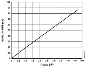
Figure 15. Gate On Time vs. Timer Capacitance, During Current Limiting Condition
