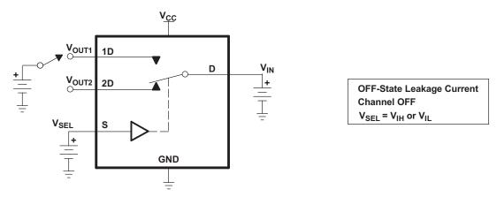
Figure 11. OFF-State Leakage Current
