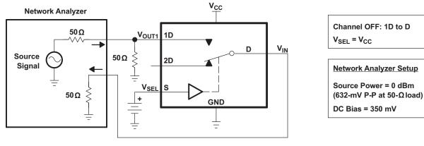
Figure 5. OFF Isolation (O<sub>ISO</sub>)
