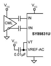
Figure 8. AC-Coupled CML Input Interface
