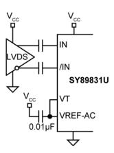
Figure 10. AC-Coupled LVDS Input Interface
