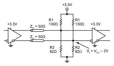
Figure 11. Parallel Termination – Thevenin Equivalent
