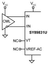
Figure 7. DC-Coupled CML Input Interface
