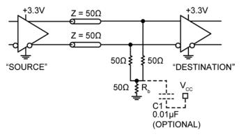
Figure 12. Three-Resistor "Y-Termination"
