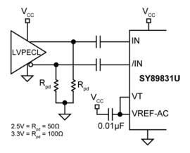
Figure 6. AC-Coupled LVPECL Input Interface
