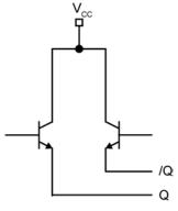
Figure 4. Simplified LVPECL Output Stage
