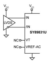
Figure 9. DC-Coupled LVDS Input Interface
