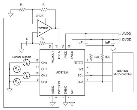
NOTE:  $f_{-3dB}$  BW = 159 kHz, R = 1 k $\Omega$ , and C = 1 nF where R = R<sub>MUX</sub> + R<sub>SENSOR</sub> + R<sub>X</sub>, and R<sub>MUX</sub> is approximately 60  $\Omega$ . Gain = 1 + R<sub>1</sub> / R<sub>2</sub>.
