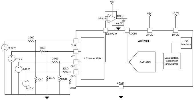
Figure 62. 0-V to 10-V Input DAQ Circuit
