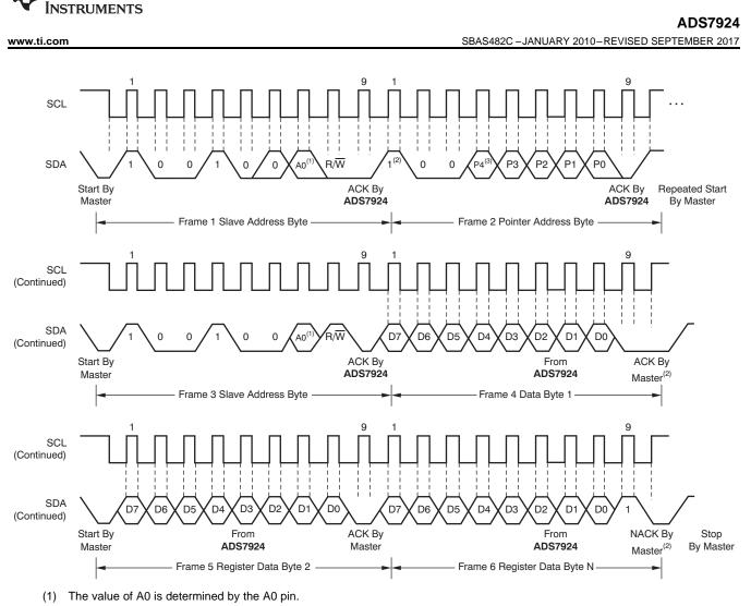
(2) When INC is set to '1', the address pointer automatically increments for multiple register reads.
