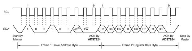
(1) The value of A0 is determined by the A0 pin.
