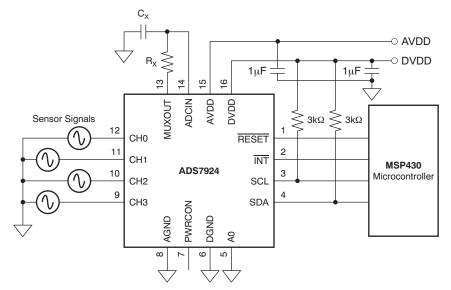
NOTE:  $f_{-3dB}$  BW = 159 kHz, R = 1 k $\Omega$ , and C = 1 nF where R = R<sub>MUX</sub> + R<sub>SENSOR</sub> + R<sub>X</sub>, C = C<sub>X</sub> + C<sub>ADCIN</sub>, R<sub>MUX</sub> is approximately 60  $\Omega$ , and C<sub>ADCIN</sub> is approximately 15 pF.
