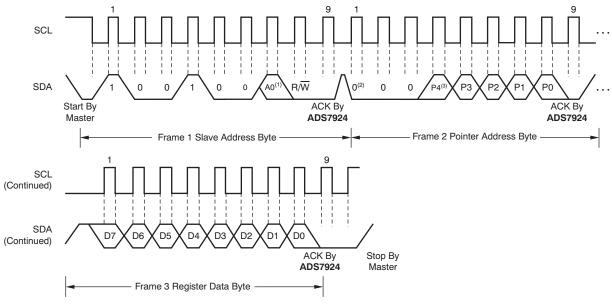
(1) The value of A0 is determined by the A0 pin.
