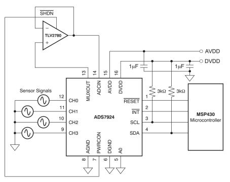
Figure 57. Sensor Data Acquisition With TLV2780 Buffer Amplifier
