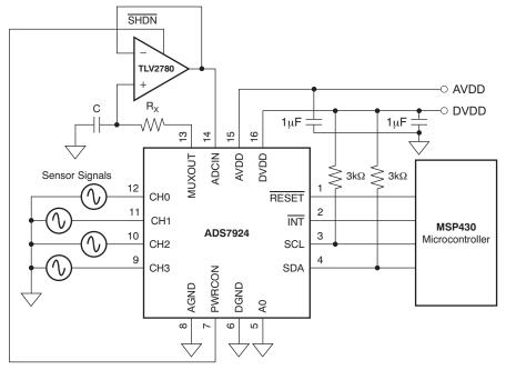
NOTE:  $f_{-3dB}$  BW = 159 kHz, R = 1 k $\Omega$ , and C = 1 nF where R = R<sub>MUX</sub> + R<sub>SENSOR</sub> + R<sub>X</sub>.
