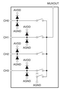
(1) See the *PWRCONFIG: Power-Up Configuration Register* register in the *Register Map* section.
