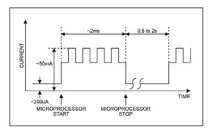
In the standby mode, the microprocessor consumes only around 200 $\mu$ A. Since the phone stays in standby for the longest percentage of time, using a 40 $\mu$ A quiescent current LDO, instead of 140 $\mu$ A, saves 100 $\mu$ A and extends the standby time by 340 $\mu$ A/240 $\mu$ A, or 1.417 times.
