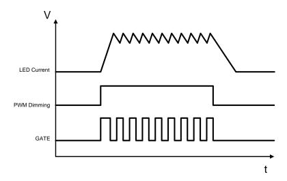
The rising and falling edges are limited by the current slew rate in the inductor. The first switching cycle is terminated upon reaching the 277mV (VDIM • 0.185) level at CS. The circuit is further reaching its steady-state within 1 switching cycles regardless of the switching frequency.
