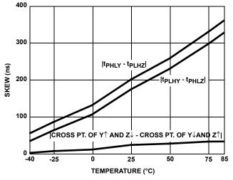
FIGURE 11. DRIVER SKEW vs TEMPERATURE (ISL8483E)
