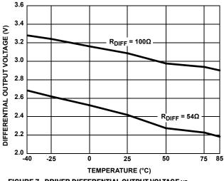
FIGURE 7. DRIVER DIFFERENTIAL OUTPUT VOLTAGE vs **TEMPERATURE**
