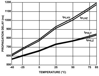
FIGURE 10. DRIVER PROPAGATION DELAY vs TEMPERATURE (ISL8483E)
