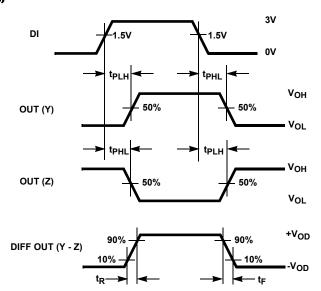
SKEW =  $|t_{PLH} (Y \text{ or } Z) - t_{PHL} (Z \text{ or } Y)|$
