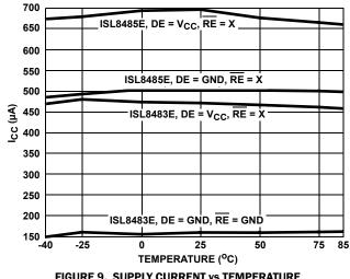
FIGURE 9. SUPPLY CURRENT vs TEMPERATURE
