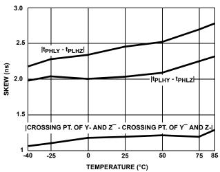
FIGURE 13. DRIVER SKEW vs TEMPERATURE (ISL8485E)
